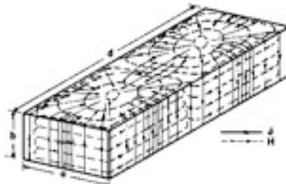
Electromagnetic field configurations in a TE<sub>102</sub> mode rectangular resonant cavity of dimensions a, b, and d.
