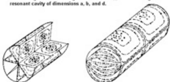
Diagrammatic sketch of the TE<sub>012</sub> (left) and TE<sub>112</sub> (right) cylindrical resonant cavity modes.
