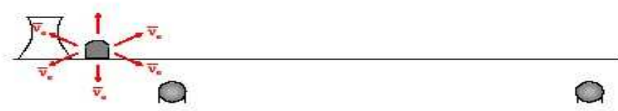
Figure 4: Schematic layout of a two detector reactor neutrino oscillation experiment.
