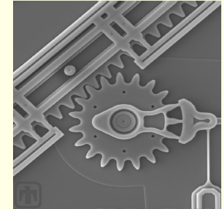
micromechanical device: pieces stick friction, levitation
